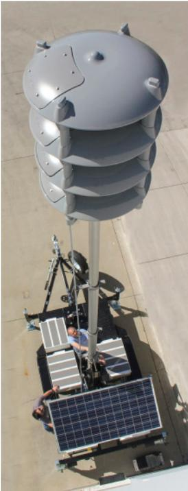
Based on Federal Emergency Management Agency (FEMA) and U.S. Military United Facilities Criteria (UFC) guidelines, the minimum standard for high-powered speaker array mass notification systems is a 0.5 Speech Transmission Index (STI) measurement.
